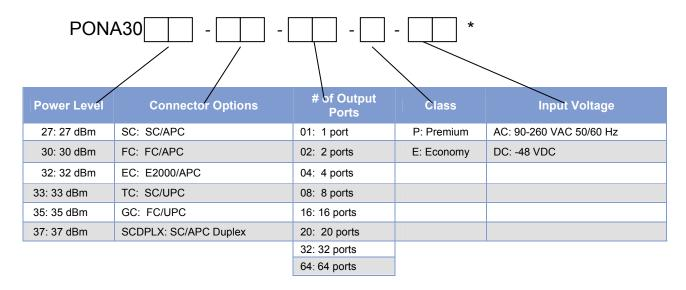
Class: Premium: Utilizes cooled pump lasers Economy: Utilizes uncooled pump lasers
